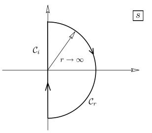
As s traverses the Nyquist path in s, then we plot a polar plot of  $F = G_0C$ . Actually we shift the origin to "-1" so that encirclements of -1 count the zeros of  $G_0C + 1$  in the right half plane.
