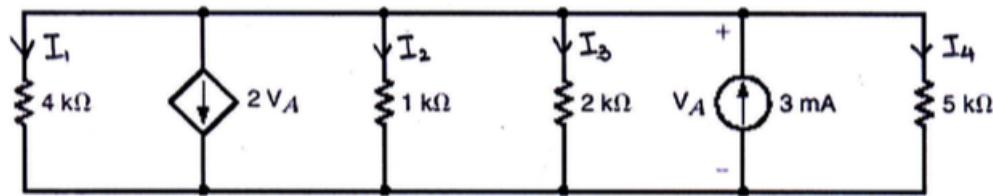
$$\text{KCL: } 3m = I_1 + 2V_A + I_2 + I_3 + I_4$$
