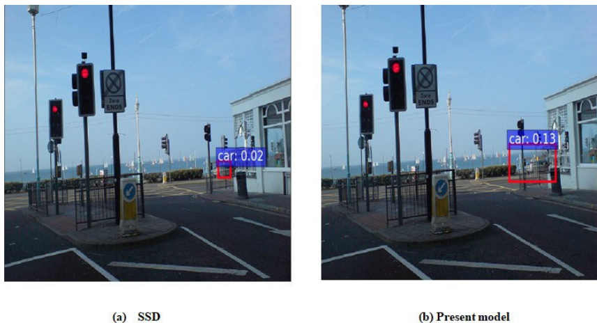
FIGURE 7. (Color online) Detection results for a covered object generated by low-level feature maps. Here, the left panel shows the result corresponding to layer conv4_3 in SSD, and result corresponding to layer Deconv2 in the present model is provided in the right panel.
