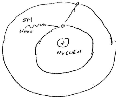
A CLASSICAL MODEL ~~AND~~ OF ATOMS, ELECTRONS ORBIT AROUND THE NUCLEUS. IF THE AN ELECTRON ABSORBS EM WAVE, IT GOES TO A HIGHER ORDER STATE (OF HIGHER ENERGY). THUS, THE ENERGY OF THE EM WAVE IS TRANSFERRED TO THE ATOMIC SYSTEM & THE EM WAVE IS ATTENUATED. AS A REVERSE PROCESS, THE ELECTRON IN THE EXCITED STATE COULD EMIT EM WAVES & THEREBY, AMPLIFIES THE EXISTING EM WAVE. ~~AND~~ THIS IS CALLED STIMULATED EMISSION & OCCURS IN LASERS. HOWEVER, THIS DOES NOT HAPPEN
