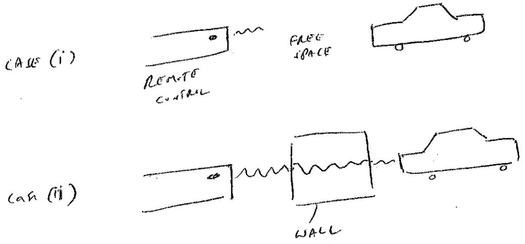
A WALL BETWEEN THE CAR & THE REMOTE CONTROL (CASE ii), THE AMPLITUDE OF THE EM WAVE AT THE CAR IS WEAKER THAN THAT IN THE CASE OF FREE SPACE (CASE i). THIS IS BECAUSE
