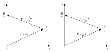
The voltage at the load as a function of time is now found by summing the voltages along the vertical line at the load position. And the same way to achieve the current in the battery.
