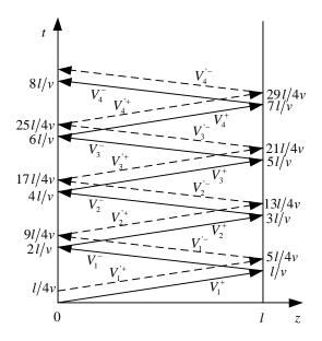
So at the load position, summing the voltage values along the vertical line, we can get the voltages for load at different time:
