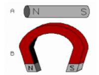
Two of the most familiar types of magnets are the bar magnet (A) and the horseshoe magnet (B). Their names reflect their physical shape.
