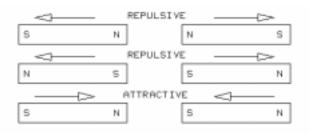
These arrows represent the direction of the attractive or repulsive magnetic forces. If a pole of one magnet is moved toward the similar pole of a second magnet (north to north or south to south), the magnets repel, or push away from, each other. If a pole of one magnet is moved toward the opposite pole of a second magnet (north to south), the magnets attract, or pull toward, each other. This relationship can be stated simply: opposite poles attract and like poles repel.
