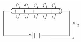
**Electromagnetism** is a form of magnetism created when current flows through a conductor. When current is present, it generates a magnetic field around the conductor similar to that of a permanent magnet. When current is removed, the magnetic field disappears.
