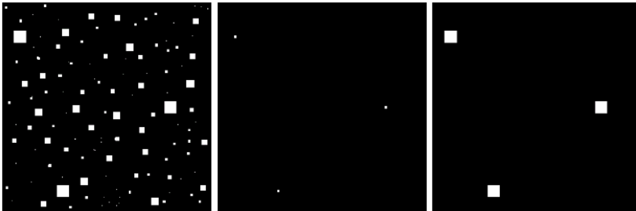
FIGURE 9.7 (a) Image of squares of size 1, 3, 5, 7, 9, and 15 pixels on the side. (b) Erosion of (a) with a square structuring element of 1's, 13 pixels on the side. (c) Dilation of (b) with the same structuring element.
