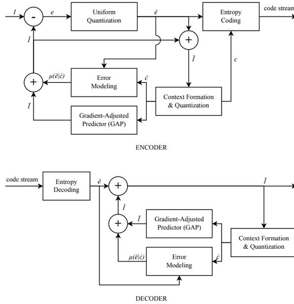
Fig. 2. Schematic description of near-lossless CALIC.
