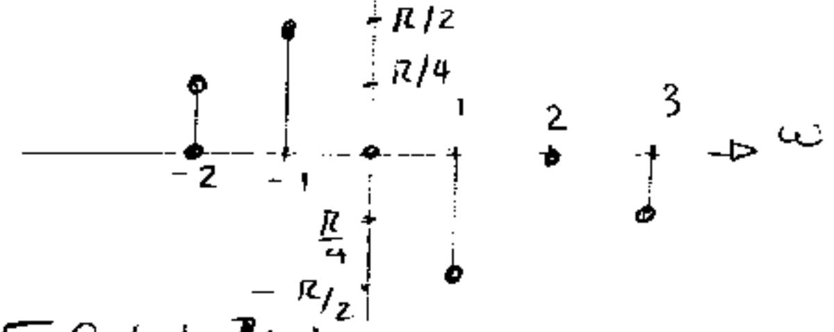
(b)  $f(t) = 3 + 4C_2(t - \pi/2) + 4\sqrt{2}C_3(3t - \pi/4)$
