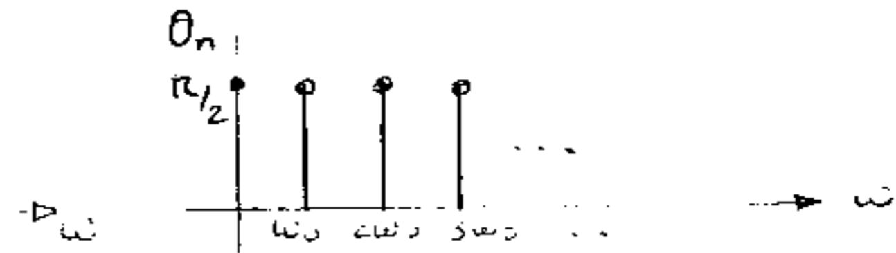
(d)  $f(t) = \frac{4}{\pi^2} \sin 2t + \frac{1}{\pi} \sin 4t - \frac{4}{9\pi^2} \sin 6t - \frac{1}{2\pi} \sin 8t + \dots$  odd signal
