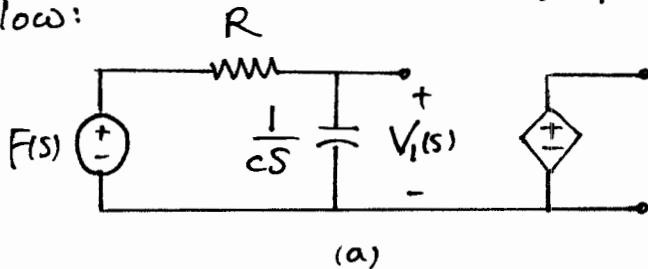
$$V_o(s) = KV_1(s) = K \frac{1}{Cs} R + \frac{1}{Cs} F(s) = \frac{Ka}{s+a} \quad a = \frac{1}{RC}$$
