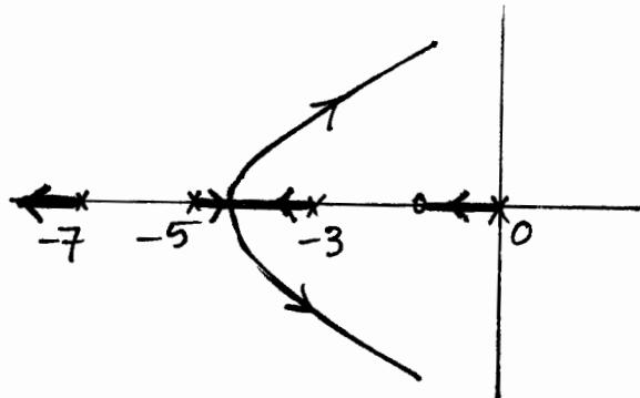
(c) The open loop poles are at 0, -3. Hence there are two root loci starting at 0 and -3 (when  $K=0$ ). Moreover the entire real axis in the LHP except the segment from -3 to -5 is a part of the root locus. There is only one open loop zero at -5. Hence one locus will terminate at -5 (when  $K=\infty$ ). The other branch terminate at  $\infty$  (when  $K=\infty$ ) along asymptote at angles  $\frac{K\pi}{n-m} = \pi$ .
