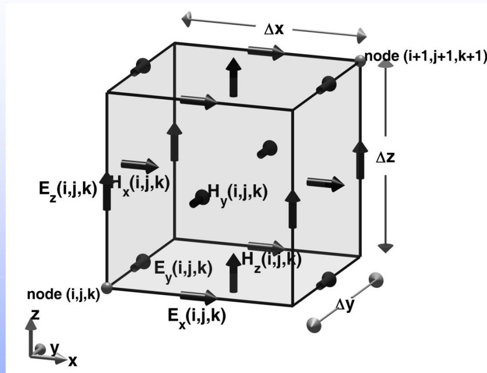
electric field vector components are placed at the centers of the edges of the Yee's cell
