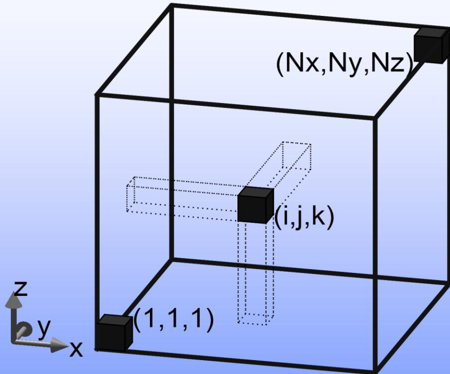
the domain is discretized into a grid of  $(N_x \times N_y \times N_z)$  cells
