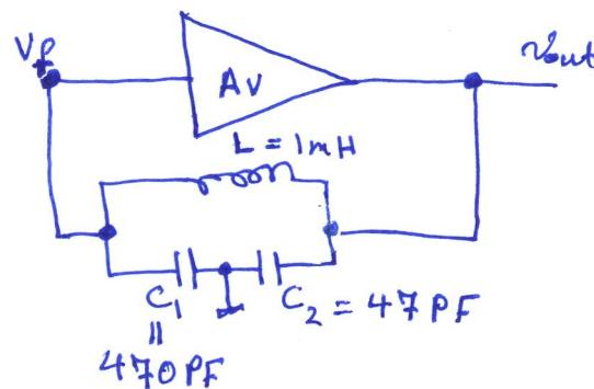
of attenuation,  $B = -\frac{C_2}{C_1} = -\frac{47 \text{ PF}}{470 \text{ PF}} = -0.1$
