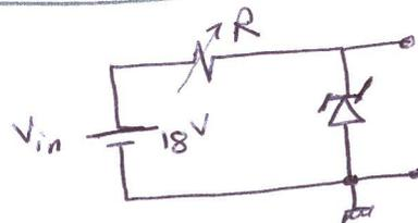
$$\therefore I_Z = \frac{V_{in} - V_Z}{R} \quad \therefore R = \frac{V_{in} - V_Z}{I_Z} = \frac{18 - V_Z(40 \text{ mA})}{40 \text{ mA}}$$
