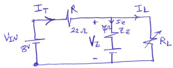
$\therefore I_L = I_T - I_Z \quad \therefore I_{L|min} = I_T - I_{Z|max}$
