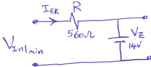
$$\begin{aligned} \therefore V_{In|min} &= I_{ZK} R + V_Z \\ &= (1.5 \text{ mA})(560) + 14 \\ &= 1.5 \times 10^{-3} \times 560 + 14 \end{aligned}$$
