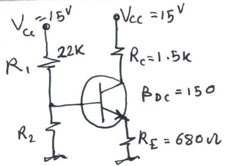
$$V_{TH} = \frac{V_{cc} R_2}{R_1 + R_2} = \frac{V_{cc}}{R_1} \left( \frac{R_1 R_2}{R_1 + R_2} \right) = V_{cc} \frac{R_{TH}}{R_1}$$
