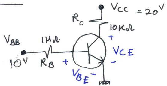
$$\therefore V_{BB} = V_{BE} + I_B R_B$$
