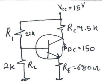
$$\therefore V_{TH} = I_E R_E + V_{BE} + I_B R_{TH}$$
