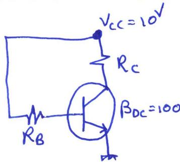
$$\therefore V_{CE} = V_{CC} - I_c R_C$$
