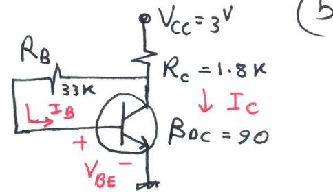
$$\begin{aligned} \therefore V_{CC} &= (I_C + I_B)R_C + I_B R_B + V_{BE} \\ &\approx I_C R_C + \frac{I_C}{\beta_{DC}} R_B + V_{BE} \end{aligned}$$
