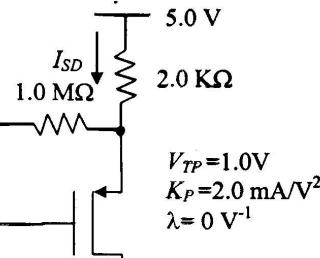
$$I_{SD} = \frac{K_P}{2} (V_{SG} + V_{TP})^2 \\ = 1.0 \times 10^{-3} (1)^2 = 1.0 \text{ mA}$$
