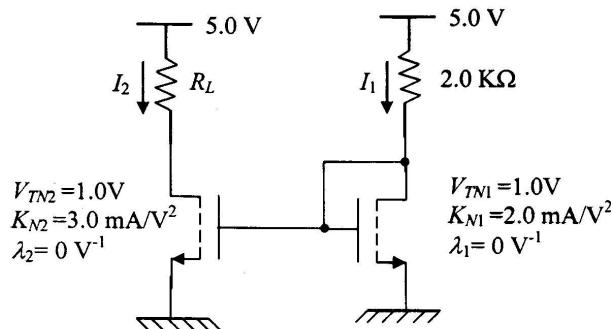
~~A<sub>2</sub>~~  $\frac{5 - V_{GS}}{2.0 \text{ k}} = \frac{K_N}{2} (V_{GS} - V_{TN})^2$
