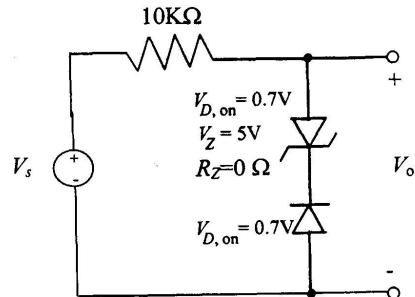
for positive voltage both diodes are off and  $V_{o,\max} = 10 \text{ V}$
