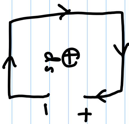
Time Varying magnetic field generates a Space varying electric field!
