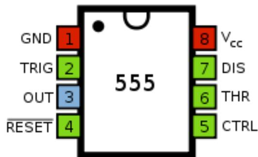
Figure 1: The pins of a 555 chip.
