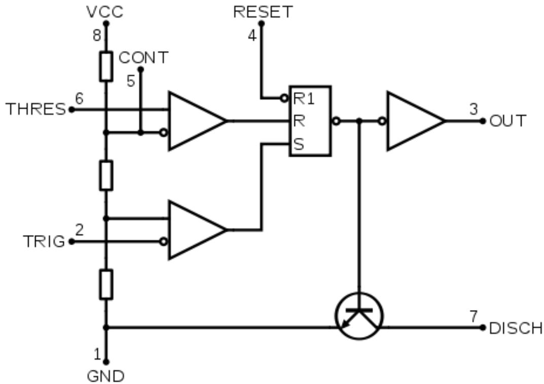
**Figure 2: Functional circuit layout of a 555 chip.**
