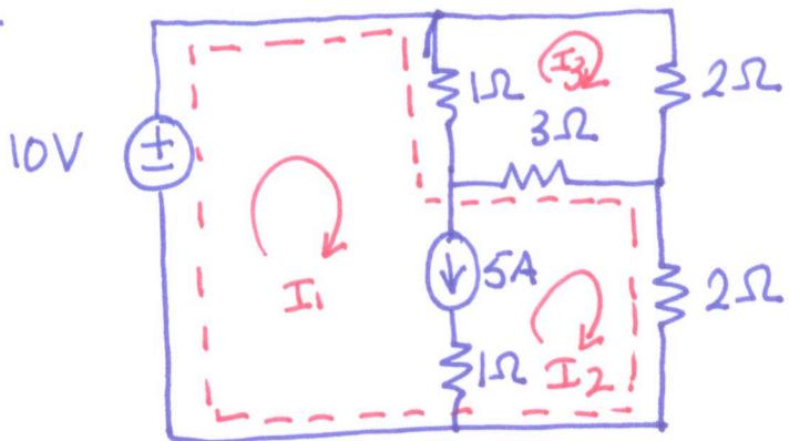
$$\text{KVL around supermesh} \quad -10 + 1(I_1 - I_3) + 3(I_2 - I_3) + 2I_2 = 0$$
