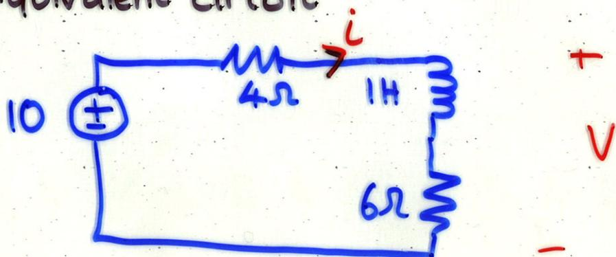
Since the source is constant, in steady state there is no voltage drop over inductor
