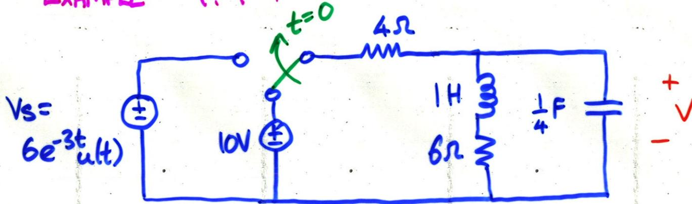
Find  $v(t)$  for  $t > 0$ , assuming circuit is in steady state at  $t=0$ .
