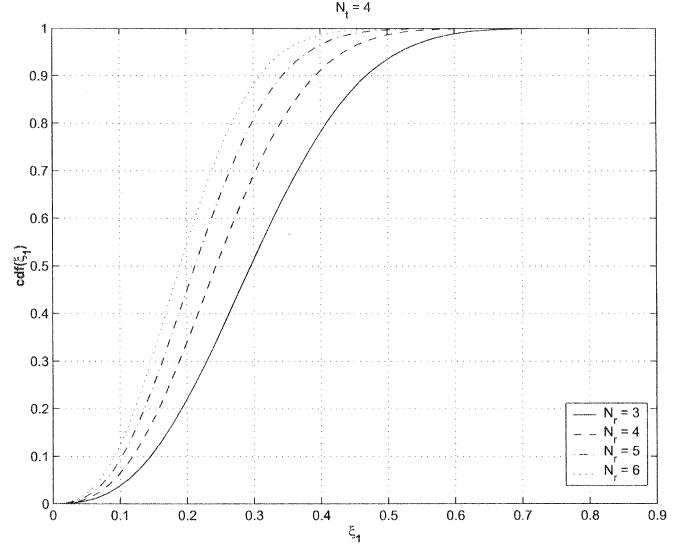
Fig. 3. cdf of  $\xi_1$  for Rayleigh fading channels.
