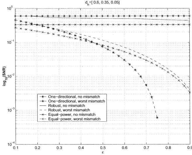
Fig. 5. SNR of conventional, robust, and omnidirectional beamformers versus the norm of error matrix.
