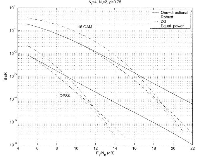
Fig. 8. SER versus  $E_s/N_0$  for a Rayleigh fading channel and delayed feedback with correlation coefficient  $\rho = 0.75$ .
