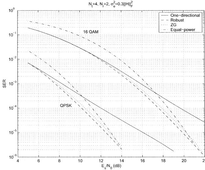
Fig. 10. SER versus  $E_s/N_0$  for a Rayleigh fading channel and Gaussian channel uncertainty with variance  $\sigma_e^2 = 0.3\|\mathbf{H}\|_F^2$ .
