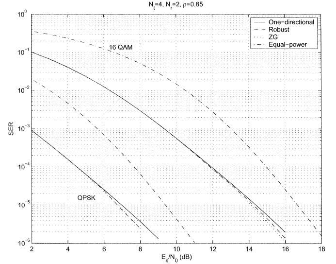
Fig. 12. SER versus  $E_s/N_0$  for a Rician fading channel with  $K = 1$  and delayed feedback with correlation coefficient  $\rho = 0.85$ .
