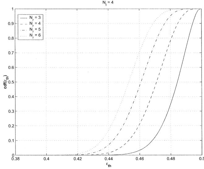
Fig. 2. cdf of  $\epsilon_{\text{th}}$  for Rayleigh fading channels.
