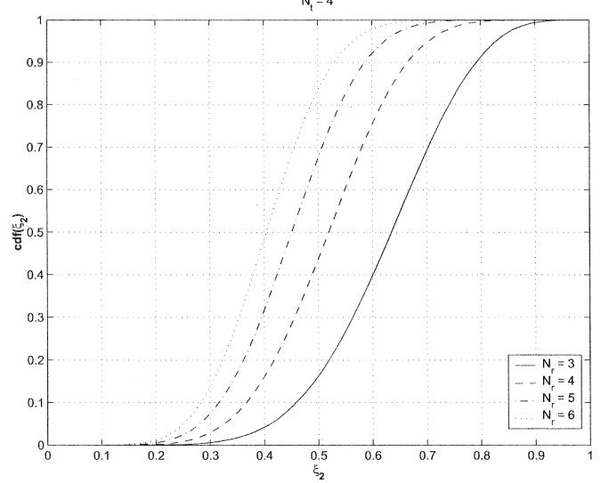
Fig. 4. cdf of  $\xi_2$  for Rayleigh fading channels.
