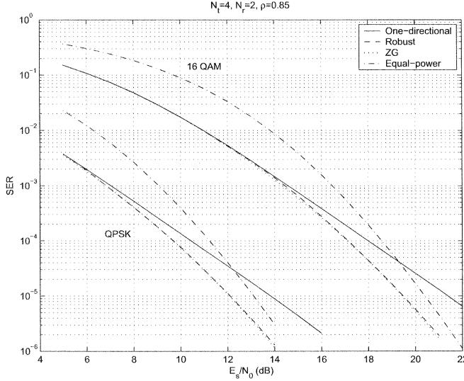
Fig. 7. SER versus  $E_s/N_0$  for a Rayleigh fading channel and delayed feedback with correlation coefficient  $\rho = 0.85$ .
