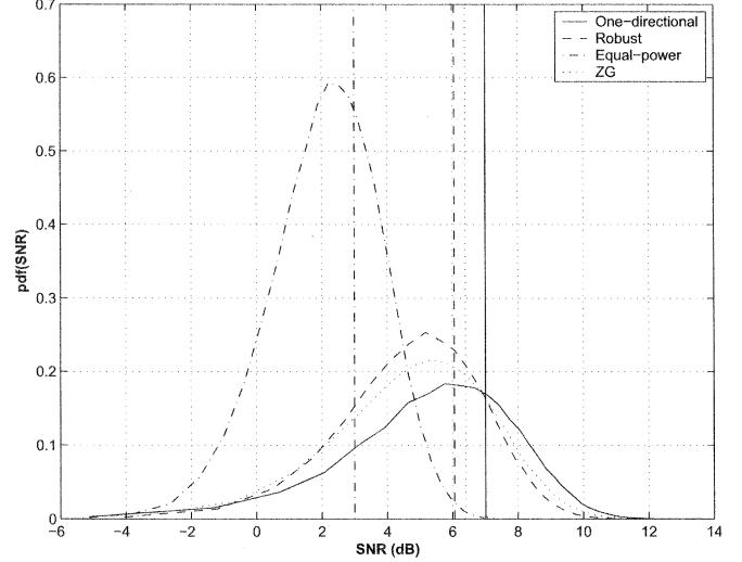
Fig. 9. SNR pdf for a Rayleigh fading channel and delayed feedback with correlation coefficient  $\rho = 0.85$ .
