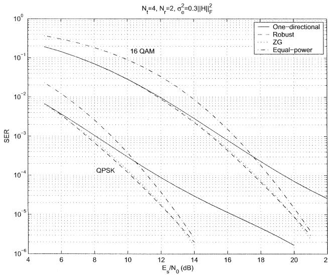
Fig. 11. SER versus  $E_s/N_0$  for a Rayleigh fading channel and uniform channel uncertainty with variance  $\sigma_e^2 = 0.3\|\mathbf{H}\|_F^2$ .
