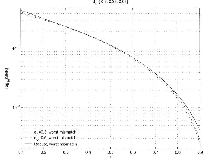
Fig. 6. Worst-case SNR for the proposed robust beamformer with precise design value for  $\epsilon$  and fixed design values for  $\epsilon_t$ .
