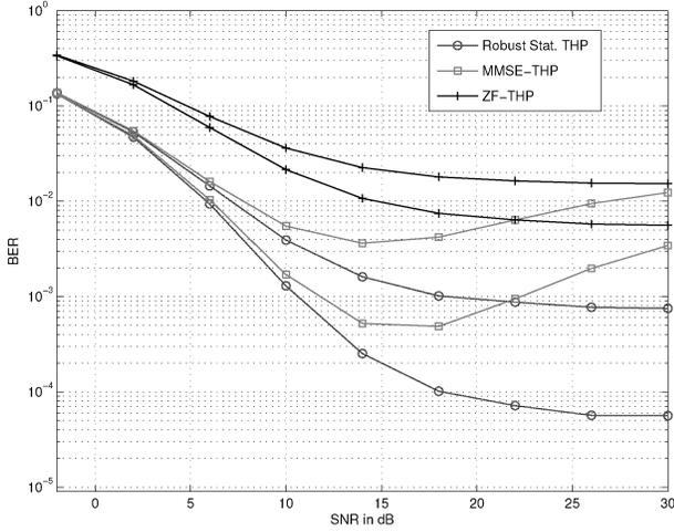
Fig. 4. Comparison between the performance of the proposed statistically robust Tomlinson-Harashima transceiver, zero-forcing Tomlinson-Harashima transceiver design (ZF-THP) in [3], [4], and the MMSE Tomlinson-Harashima transceiver design (MMSE-THP) in [5] for values of channel uncertainty  $\epsilon^2 = 0.05, 0.1$  for a system with  $N_t = 4$  and  $K = 4$  using QPSK signalling. The upper performance curve of each method corresponds to channel uncertainty  $\epsilon^2 = 0.1$ .
