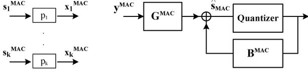
Fig. 3. The Dual MAC with decision feedback equalization.
