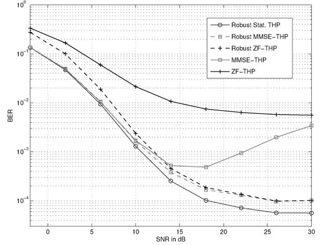
Fig. 5. Comparison between the performance of the proposed statistically robust TH transceiver, zero-forcing TH transceiver design (ZF-THP) in [3], [4], and the MMSE TH transceiver design (MMSE-THP) in [5], robust zero-forcing TH (Robust ZF-THP) approach introduced in [10], and the robust MMSE Tomlinson-Harashima (Robust MMSE-THP) approach introduced in [9], for values of channel uncertainty  $\epsilon^2 = 0.05$  for a system with  $N_t = 4$  and  $K = 4$  using QPSK signalling.
