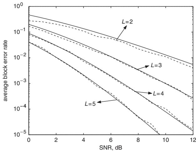
**Fig. 1** Simulated average block error rate (dashed) and the theoretic approximation to the average block error probability (solid) for optimally precoded schemes for frequency-selective fading channels of lengths  $L=2, 3, 4$  and  $5$
