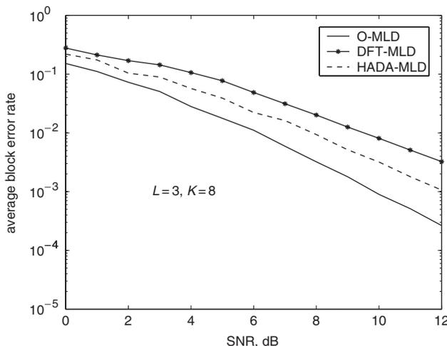
**Fig. 2** Block error rate performance comparison of the optimally precoded system (O-MLD) with systems which use the IDFT precoder (DFT-MLD) or Hadamard precoder (HADA-MLD) for the length  $L=3$  frequency-selective fading channel in example 1
