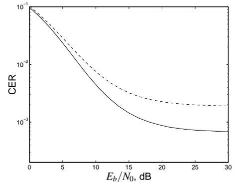
Figure 4: Simulated chip error rates (CER) against signal-to-noise ratio for Example 1. Legend—Dashed: IS95 filter; Solid: robust filter.
