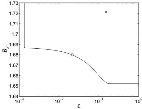
Figure 2: The trade-off between  $B_g$  and  $\epsilon$  (the bound on  $\gamma_g$ ) for the IS95 standard. The ‘ $\times$ ’ and ‘ $\circ$ ’ denote the positions achieved by the IS95 filter and the robust filter in Fig. 3(b), respectively.
