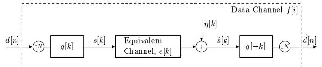
Figure 1: Discrete-time model of baseband PAM.
