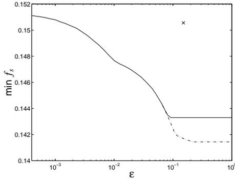
Figure 5: Minimal stopband edge,  $f_s$  against  $\epsilon$  for the IS95 mask, with (solid) or without (dash-dot) the constraint  $B_g \leq B_{\text{IS95}}$ . The ‘x’ denotes the position of the IS95 filter.
