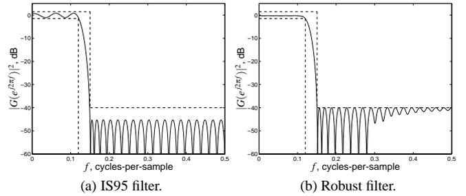
Figure 3: Relative power spectra (in decibels) of the filters in Example 1, with the spectral mask from IS95.
