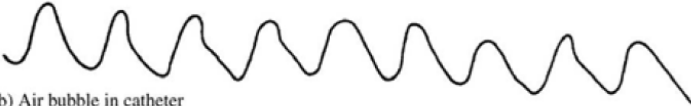
(b) Air bubble in catheter
