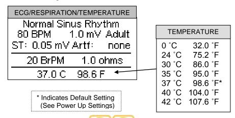
These temperatures can be selected by using to highlight the parameter to change and using to scroll to the desired option. Then is used to accept the new setting.
