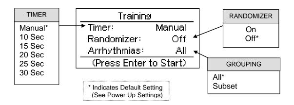
The Timer, Randomizer and Arrhythmias can be selected by using to highlight the parameter to change and using to scroll to the desired option.
