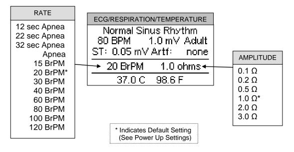
These Rates and Amplitude (Impedance Variations) can be selected by using to highlight the parameter to change and using to scroll to the desired option. Then is used to accept the new setting.
