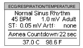
The display will count down the Apnea period and then revert to the previous BrPM setting, display and output.
