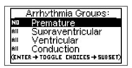
**4.** To select some of the arrhythmias in a group, use to display the list of arrhythmias for a specific group. Then use to scroll through the arrhythmias. Any arrhythmia marked with a check ( , ) will be included in the subset. Use to toggle the selection of an arrhythmia on and off.
