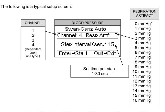
**NOTE:** In models 2220 and 2240, the unit will auto select BP based on the channel that was used to enter the mode. However, it may be changed before beginning a sequence.
