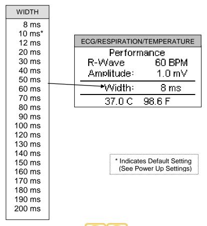
These widths can be selected by using to highlight the parameter to change and using to scroll to the desired option. Then **ENTER** is used to accept the new setting.
