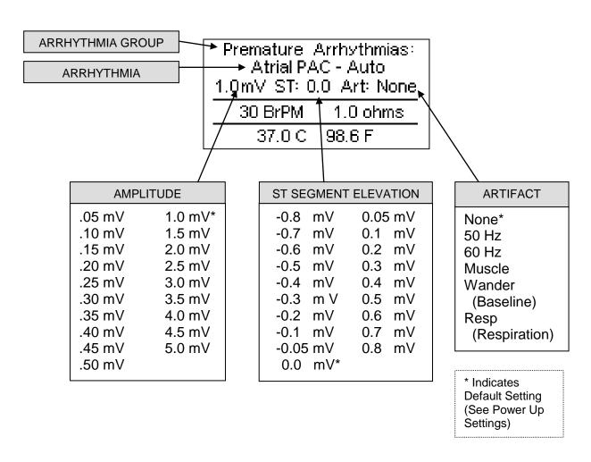
The grouping, arrhythmias and amplitude can be selected by using to highlight the parameter to change and using to scroll to the desired option.
