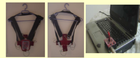
Figure 8. Front of Wearable Module (Left), Back of Wearable Module (Middle), Wireless Receiver Module (Right)
