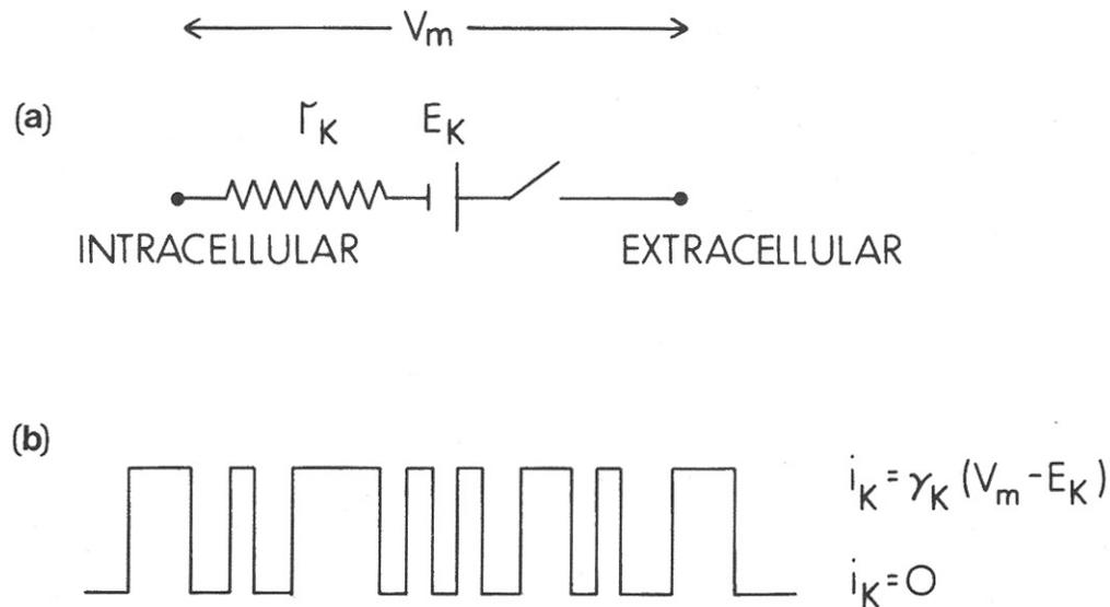
*Figure 4.7.* (a) Electrical circuit representation for a single (potassium) channel showing fixed resistance  $r_K$ , potassium Nernst potential  $E_K$ , and the transmembrane potential  $V_m$ . The closing and opening of the switch simulates the stochastic opening and closing of the channel gate. (b) Single-channel current corresponding to (a), where  $\gamma_K = 1/r_K$ . This is an idealization of the recording shown in Fig. 4.6.
