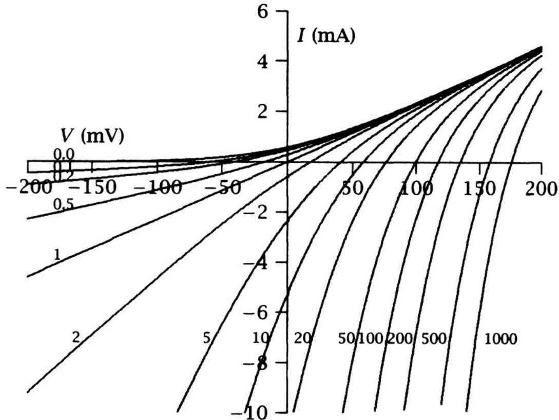
**Figure 2.5** Current-voltage relations given by equation 2.7.17 (GHK current equation) for various values of  $[C]_{out}/[C]_{in}$  (indicated by small numbers near each curve).
