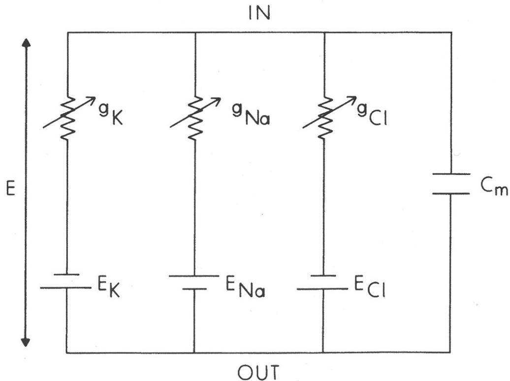
*Figure 3.3.* Parallel-conductance model of an excitable membrane, for which one assumes independent conductance channels for  $K^+$ ,  $Na^+$ , and  $Cl^-$ . The battery polarity is chosen to show that the nominal Nernst potential of  $E_K$  and  $E_{Cl}$  is negative and  $E_{Na}$  positive.
