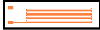
Figure 1. A strain gage may consist of a tightly wound wire.
