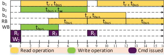
Fig. 1. An example schedule for 4 requests accessing different banks with  $t_{bus} = 4$  and  $t_r = t_w = 3$ .
