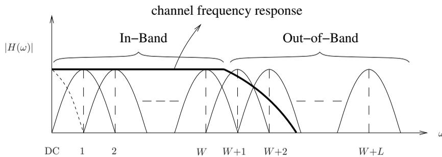
Fig. 1. Spectrum of an MSM wireless optical system using  $W$  in-band and  $L$  out-of-band carriers.
