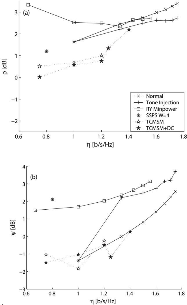
Fig. 4. In-band techniques: normalized average optical power ( $\rho$ ) (a) and normalized peak optical power ( $\psi$ ) (b) versus bandwidth efficiency ( $\eta$ ) for normal MSM, tone injection [10], You block codes [14], SSPS [17] and TCMSM. Note the prefix ‘DC’ indicates results using DC bias detection technique.
