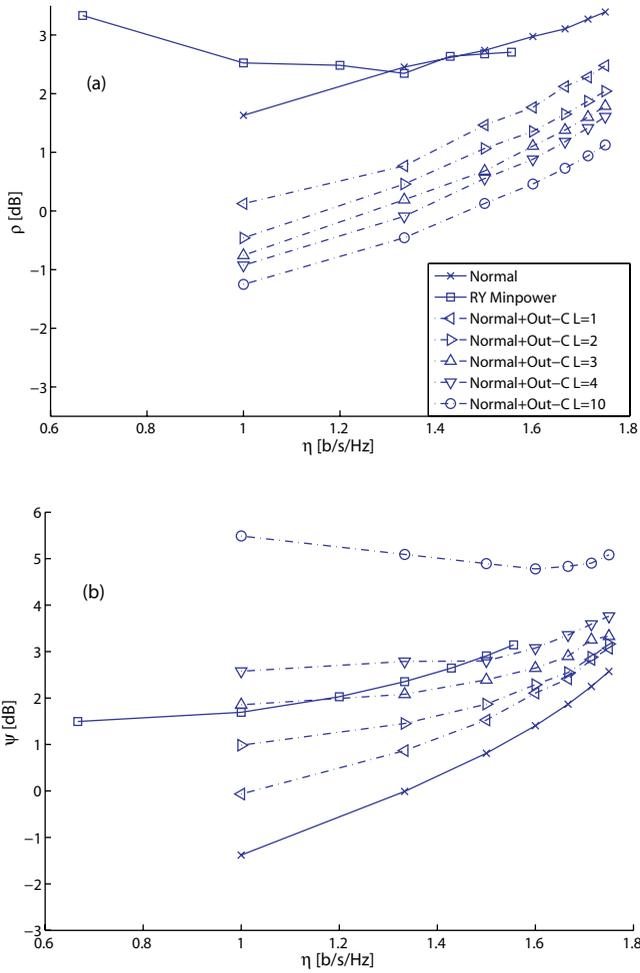
Fig. 6. Selecting  $L$ : normalized average optical power ( $\rho$ ) (a) and normalized peak optical power ( $\psi$ ) (b) versus  $\eta$  for  $L = 1, 2, 3, 4, 10$  out-of-band carriers optimized over  $C$ .
