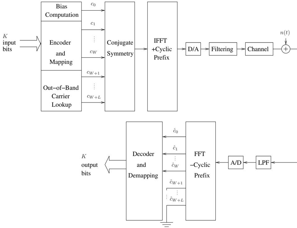
Fig. 2. MSM wireless optical system with out-of-band carriers.
