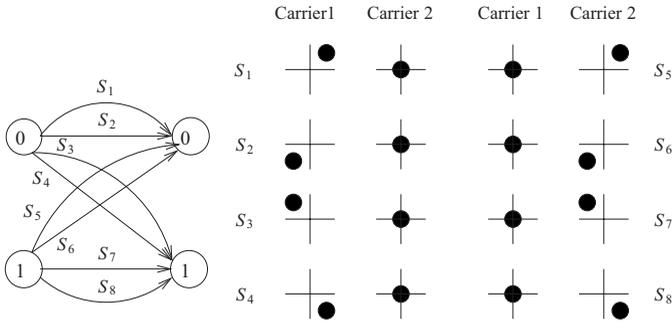
Fig. 3. Trellis structure and MSM constellation points for  $K = 2$ ,  $M = 2$ ,  $W = 2$  and  $U = 1$ .
