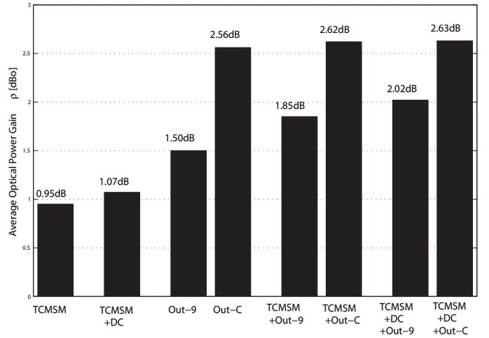
Fig. 7. Average optical power gain,  $\rho$ , over normal MSM by applying the developed techniques at  $\eta = 1$ . The label ‘TCMSM’ denotes in-band coding, ‘Out’ indicates  $L = 4$  out-of-band carriers and ‘DC’ indicates the use of the DC bias technique.
