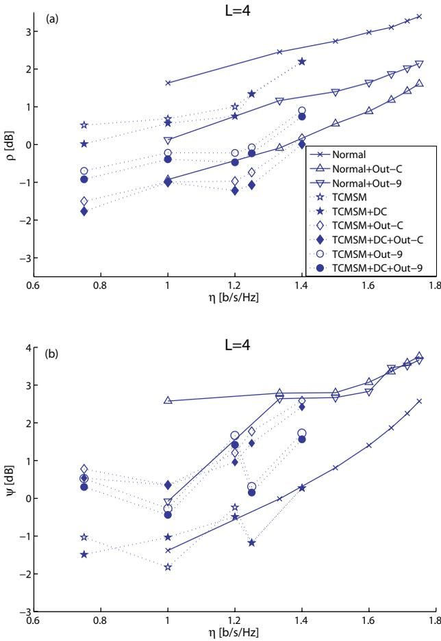
Fig. 5. Out-of-band techniques: normalized average optical power ( $\rho$ ) (a) and normalized peak optical power ( $\psi$ ) (b) versus bandwidth efficiency ( $\eta$ ) and using  $L = 4$  out-of-band carriers for normal and in-band coded (TCMSM) systems. Note that the prefix 'Out' indicates techniques using out-of-band carriers, 'C' indicates carriers selected over the complex plane and '9' indicates amplitudes were selected from scaled 9-APSK.
