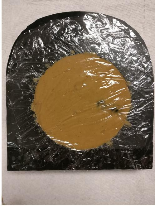
Fig. 17. The second layer of an OUT constructed from absorber sheets, a PBJ mixture, and two blueberries embedded on the side.
