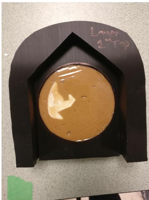
Fig. 13. An OUT constructed from absorber sheets, a PBJ mixture, and alginate embedded on the side.
