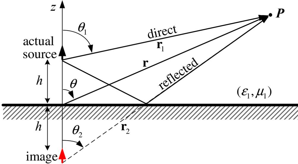
The field at the observation point  $P$  is a superposition of the fields of the actual source and the image source, both radiating in a homogeneous medium of constitutive parameters  $(\epsilon_1, \mu_1)$ . The actual (or original) source is a current element  $I_0 \Delta l$  (infinitesimal dipole). Therefore, the image source is also an infinitesimal dipole. The respective field components are:
