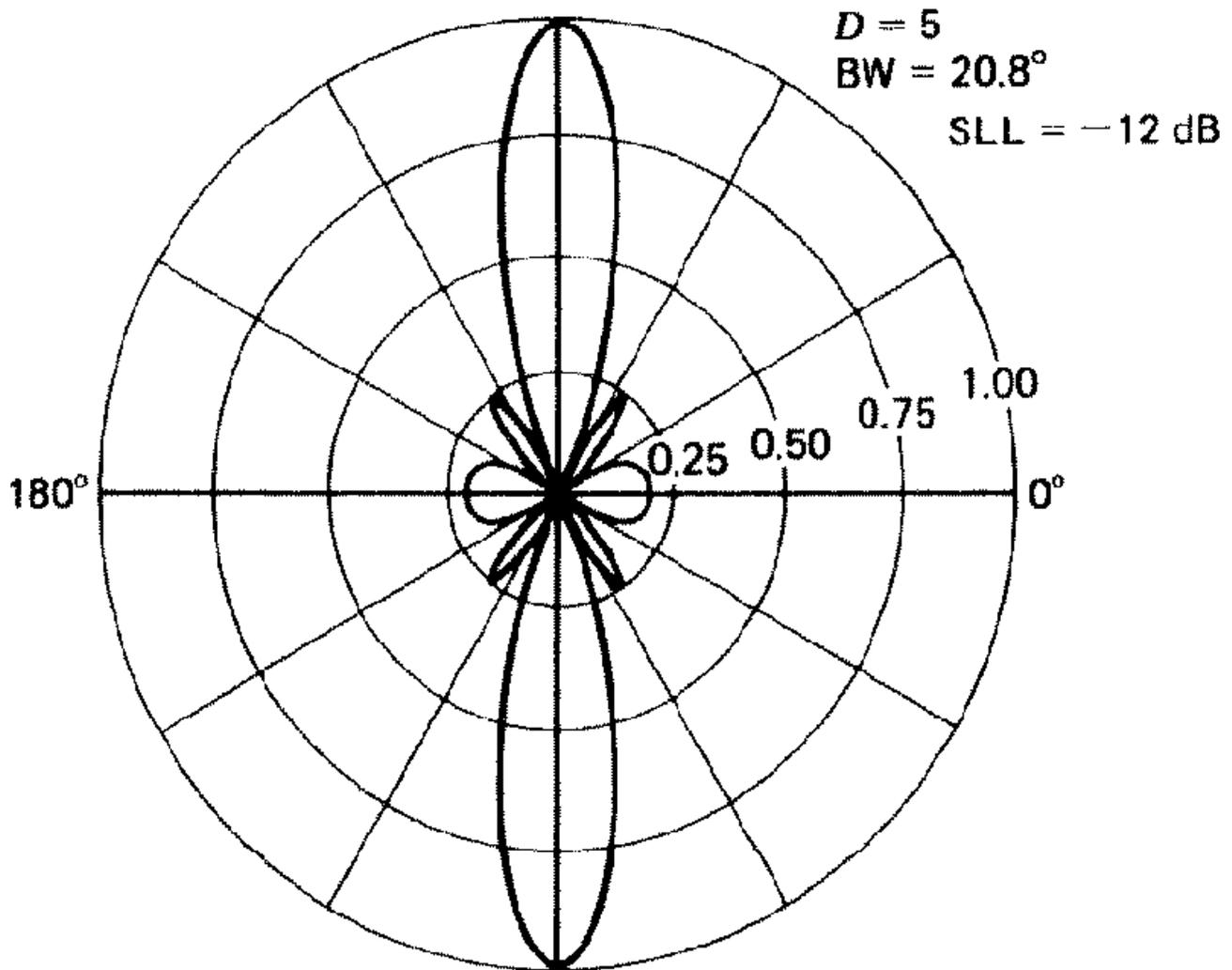
b) **triangular** (1:2:3:2:1) amplitude distribution ( $N = 5$ ,  $d = \lambda / 2$ , max. at  $\theta_0 = 90^\circ$ )
