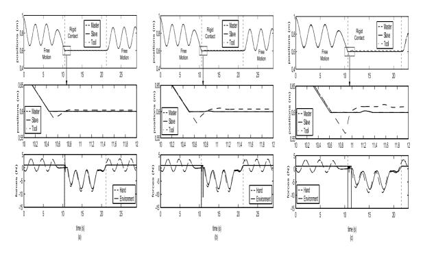
Figure 4.4: Position and force tracking in simulation for mismatched model parameters: (a) 125ms delay (b) 250ms delay (c) 500ms delay.
