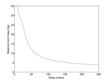
Figure 4.7: Robustness of rigid contact controller w.r.t. mismatch in arm mass  $(m_h = 0.35 \text{ in design})$ .
