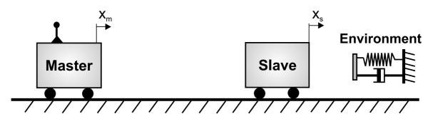
Figure 3.3: Schematic of the single-axis teleoperation system.
