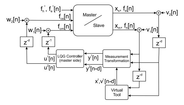
Figure 4.2: The LQG teleoperation control system.
