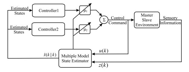
Figure 3.2: Multiple model state estimation and control for two modes.
