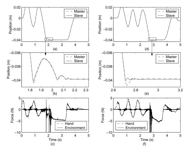
Figure 3.7: Position and force tracking in experiment: (a),(b),(c) fixed-gain controller (d),(e),(f) adaptive multi-model controller.
