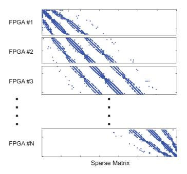
Figure 5.4: Portions of **K** matrix stored on each FPGA for performing first level of parallelization
