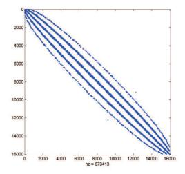
Figure 6.11: The K matrix arising from performing FE analysis on an sphere in our tests
