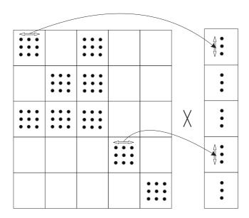
Figure 6.4: Performing sparse matrix by vector multiplication for rows 0 and 9 concurrently demands reading data from different locations of d vector
