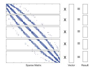
Figure 5.2: Matrix partitioning for increased parallelism. Figure from [42]
