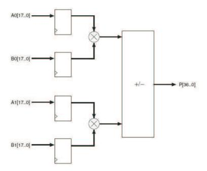
Figure 6.1: Basic two-multiplier adder building block
