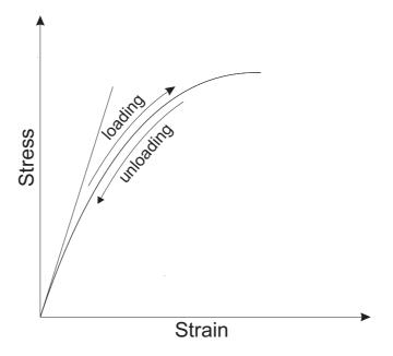
Figure 3.2: Strain-stress characteristics of a non-linear elastic material
