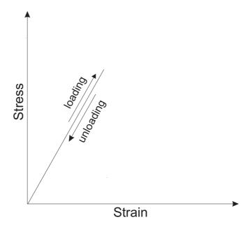
Figure 3.1: Strain-stress characteristics of a linear elastic material
