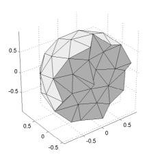
Figure 3.4: Discretizing a sphere into tetrahedron elemental shapes
