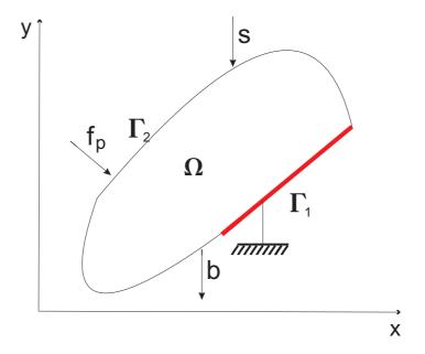
Figure 3.3: A 2D object with external possible forces applied to it. In this figure, s represents the surface traction b is the body force fp represents the point loads  $\Gamma$ 1 and  $\Gamma$ 2 refer to constraint and non-constraint nodes of domain $\Omega$ .
