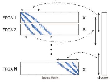
Figure 6.13: Portions of d vector needed for each FPGA for performing Kxd multiplication d vector
