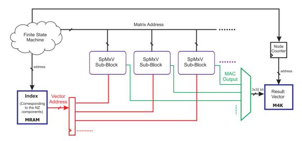
Figure 5.3: Third level of parallelization: top-view block diagram of the hardware-based sparse matrix by vector multiplication. Figure from [42]
