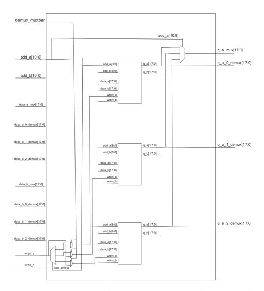
Figure 6.6: Memory architecture for one dimension (out of x, y or z) of vectors, wiring for port a (inputs and outputs with " $_{-}a$ " term in their names) has been depicted in this figure and port b has similar wirings. Ports with names including "data $_{-}$ " are input ports and those with term " $q_{-}$ " are output ports
