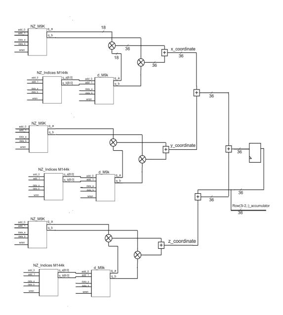
Figure 6.10: Data path for K\*d multiplication for row (3i-2,:), the same architecture exists for rows (3i-1,:) and (3i,:) for each sub-partition. In this figure, d\_M9k refers to M9ks storing **d** vector values for sub-partitions.
