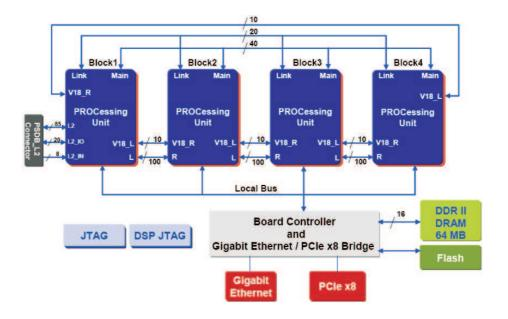
Figure 6.2: ProcStar III system block diagram [4]
