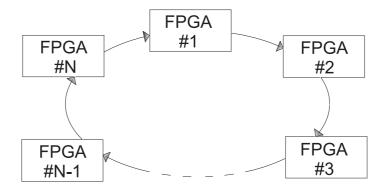
Figure 6.12: The communication scheme in multi-FPGA architecture. Arrows show the direction of the data flow.
