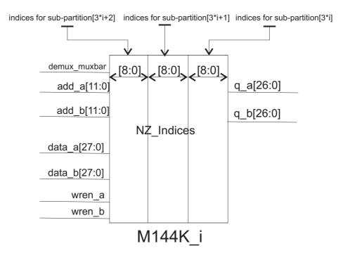
Figure 6.9: Memory architecture for  $nz\_indices$  storage in M144k rams. Ports including the term "data\_" in their names are input ports and those with "q\_" are output ports
