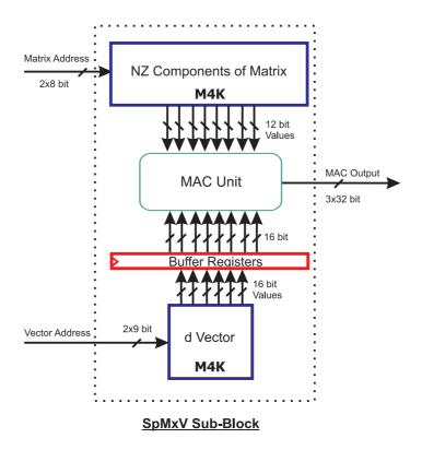
Figure 5.1: The connection of MAC units to memory blocks. Figure from [42]
