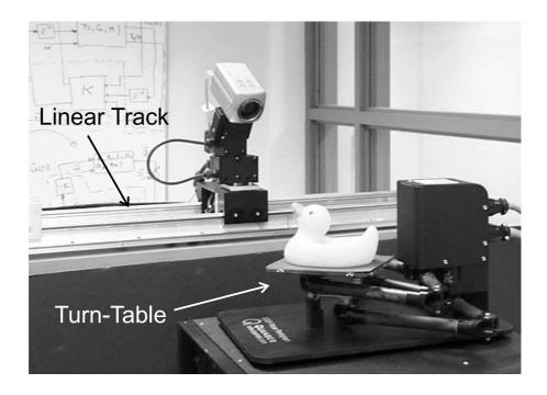
Figure 6.2: Camera 2 is positioned by a linear track; a twin pantograph unit serves as the turn-table.
