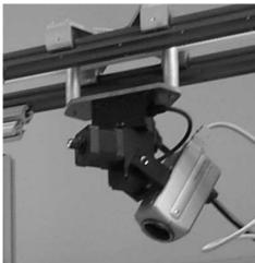
Figure 6.3: Pan-tilt units with the cameras attached; the left picture shows a sample positioning of Camera 2, whereas the picture on the right depicts the positioning of Camera 1.
