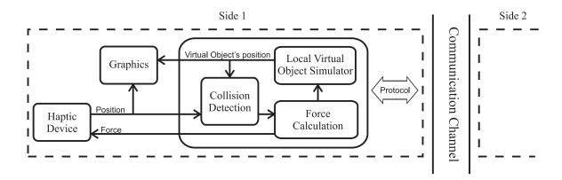
Figure 7.1: Building blocks of the multi-user distributed haptic simulator. The two sides of the communication channel are identical.
