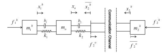
Figure 3.2: Model of centralized single-axis cooperative haptics.
