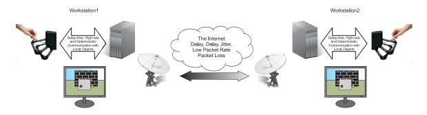
Figure 3.3: General representation of a distributed dual-user haptic system over a packet switched network.
