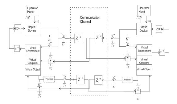
Figure 3.5: Distributed control architecture; state predictors, shown by dashed blocks, are added to improve performance.
