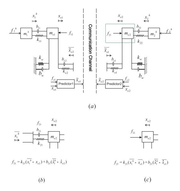
Figure 5.3: (a) The distributed architecture with state prediction. The dashed box displays the force applied to virtual object at side 2 from user at side 1. (b) Feedback scheme. (c) Feedforward scheme.
