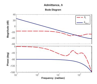
Figure 4.2: User's perceived admittance in distributed architecture  $h_1(j\omega)$  and ideal admittance  $h_{Ideal}(j\omega)$  in free motion
