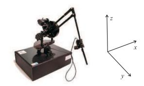
Figure 8.5: PHANTOM Premium 1.5A Haptic Device by SensAble and the coordinate frame assigned to it.
