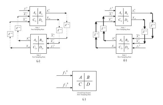
Figure 3.6: Subsystem resampling approach in modeling the distributed control architecture. (a) Constructing the state-space equations of each side at the fast sampling rate ( $T_c$ ). (b) Resampling at the slow sampling rate ( $T_t$ ). (c) Connecting the two subsystems and finding the closed-loop system dynamics. [35]
