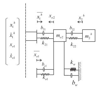
Figure A.5: Single-axis model of side2 of the two-user haptic system.
