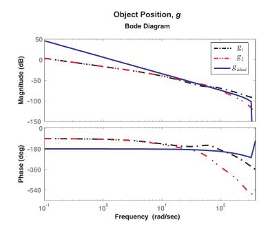
Figure 4.3: Object position  $g_i(j\omega)$  and ideal position  $g_{Ideal}(j\omega)$  in free motion
