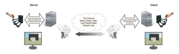
Figure 3.1: General representation of a centralized dual-user haptic system over a packet switched network.
