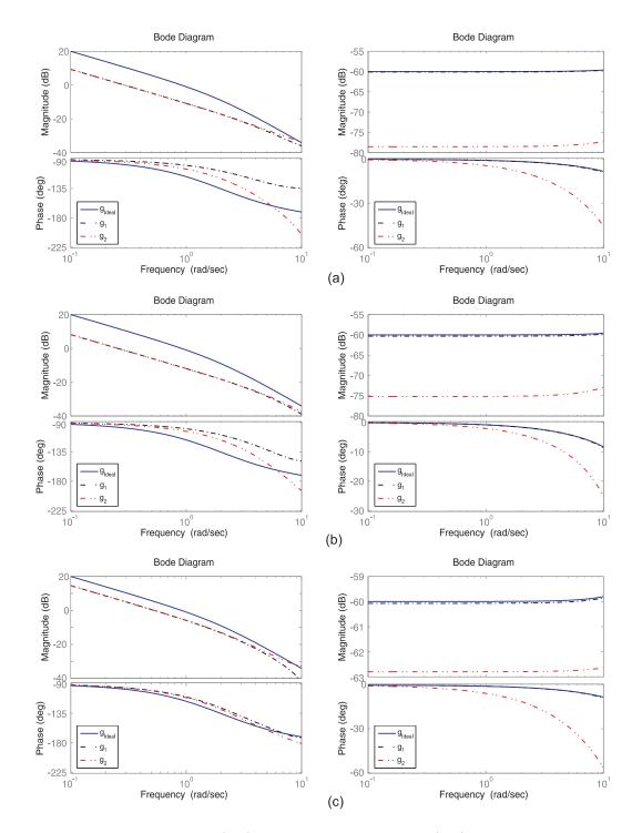
Figure 6.2: Object position  $g_i(j\omega)$  and ideal position  $g_{Ideal}(j\omega)$  in free motion (left column) and contact (right column). (a) Without prediction; (b) With prediction; (c) Feedforward + prediction.
