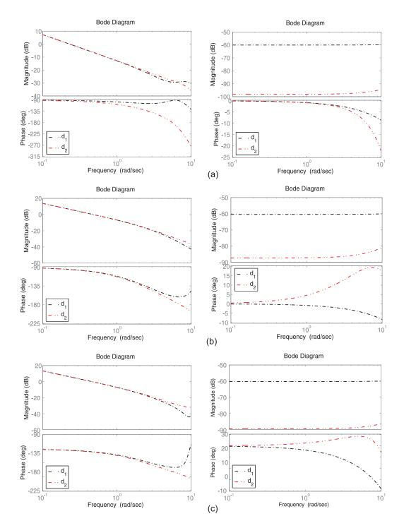
Figure 6.3: Response to disturbance  $d_i(j\omega)$  in free motion (left column) and contact (right column). (a) Without prediction; (b) With prediction; (c) Feedforward + prediction.
