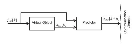
Figure 5.1: Predictor- Block diagram representation.
