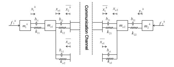
Figure 3.4: Model of distributed single-axis cooperative haptics.
