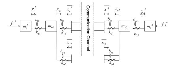
Figure A.1: Model of distributed single-axis cooperative haptics.
