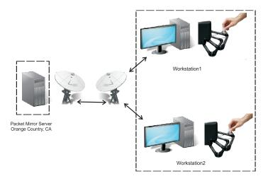
Figure 7.3: Experiment network setup. Icons from http://www.devcom.com/.
