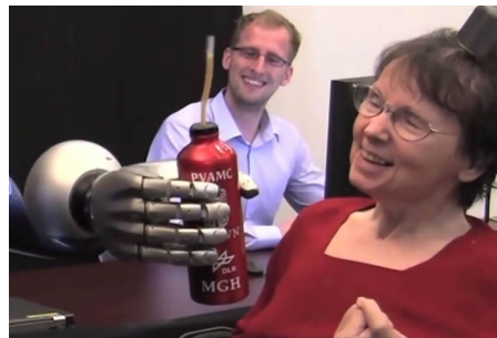
Woman controls robotic arm with 100-channel Utah array [2]
