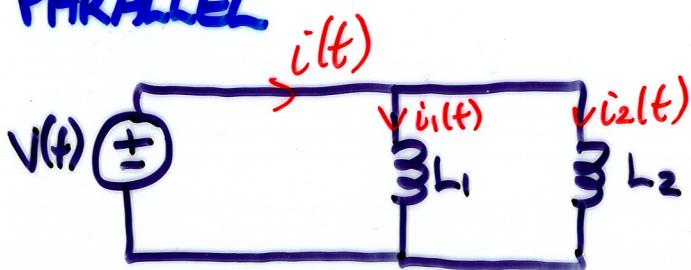
$$i_k(t) = i_2(t_0) + \frac{1}{L_2} \int_{t_0}^t v(x) dx$$
