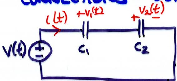
$$v_i(t) = v_i(t_0) + \frac{1}{c_i} \int_{t_0}^t i(x) dx$$
