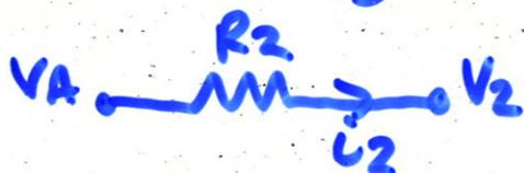
$\frac{V_A - V_2}{R_2} = i_2$ .
