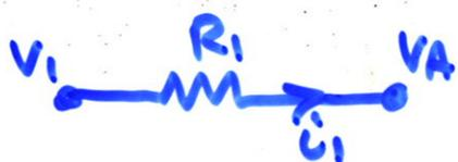
Ohm's Law  $\frac{V_1 - V_A}{R_1} = i_1$
