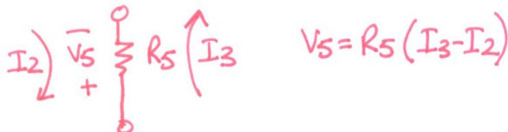
$$V_5 = R_5 (I_3 - I_2)$$
