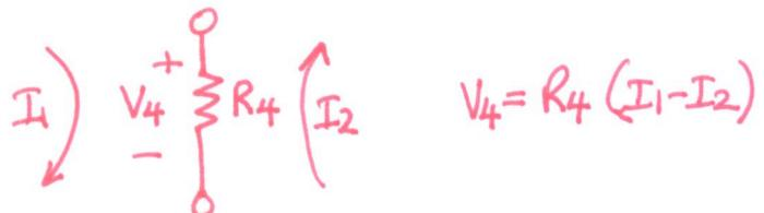
$$V_4 = R_4 (I_1 - I_2)$$
