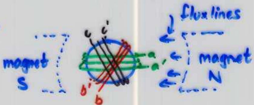
Note that the coils cut the flux lines  $120^\circ$  apart, + hence produce voltages which are separated by  $\approx 120^\circ$  in phase
