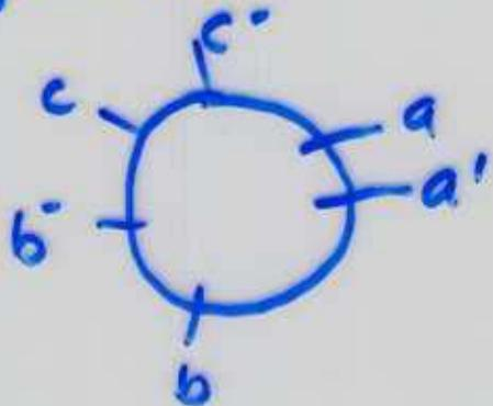
One way is to connect all the "dashed" terminals together to form a "neutral" terminal.
