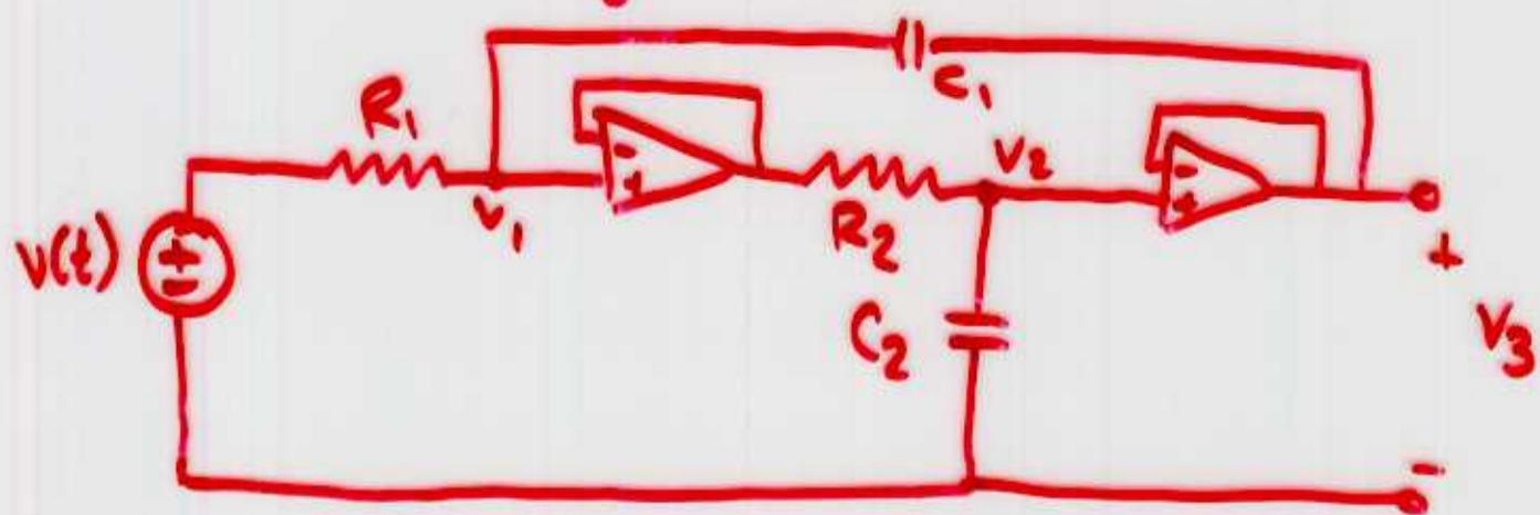
$$H(s) = \frac{v_3(s)}{v(s)} = \frac{\omega_0^2}{s^2 + (\frac{1}{R_1 C_1}) s + \omega_0^2}$$
