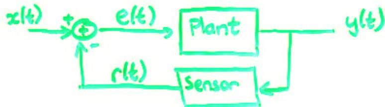
Plant : acts on "error signal"  $e(t)$  to produce output  $y(t)$
