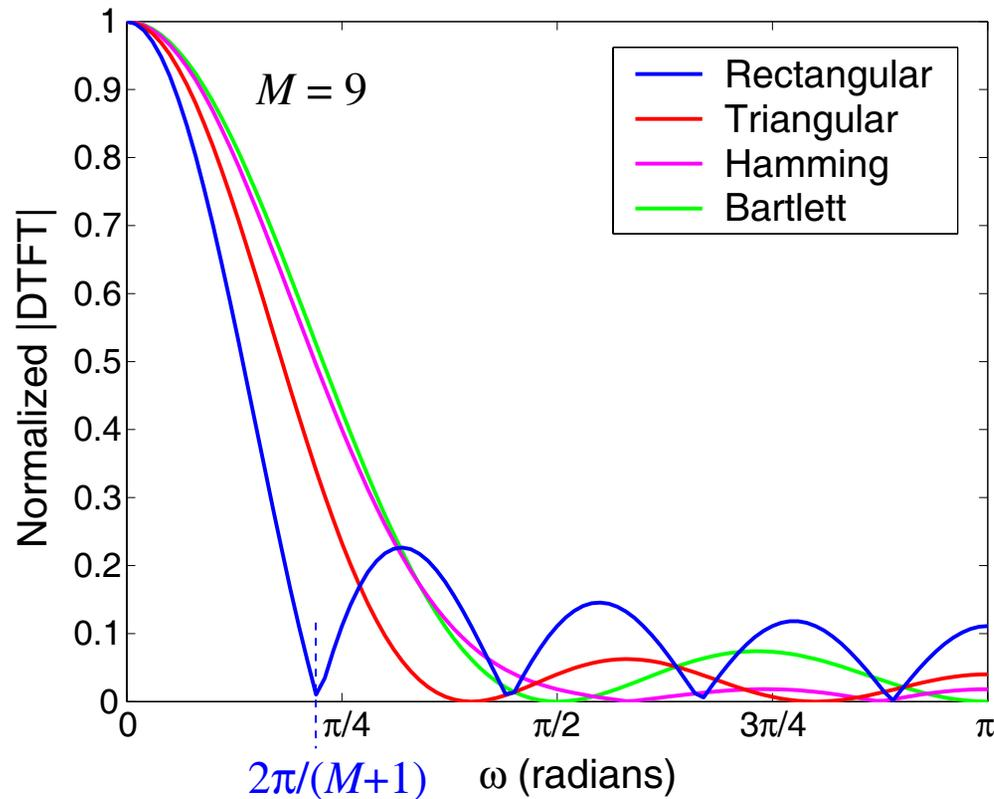
From the shape of the rectangular window's spectrum, it is reasonable to assume that we should be able to resolve two frequency components that are separated by approximately half the mainlobe width, i.e.,  $2\pi/(M+1)$ .
