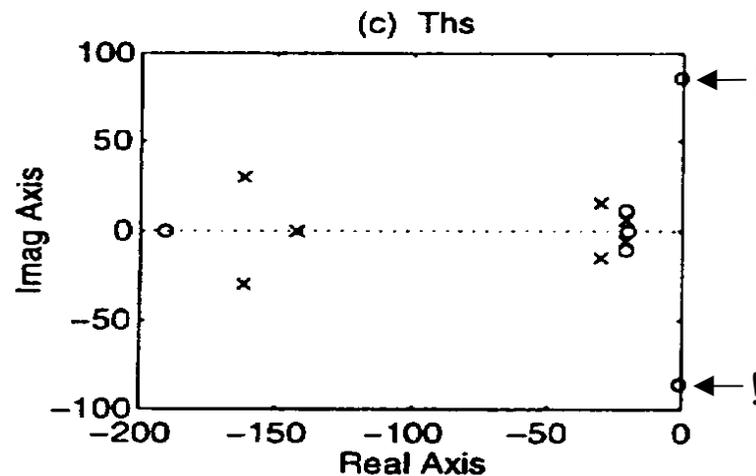
The corresponding frequency response shows a dip at the frequency of the imaginary axis zeros (*see next slide*).
