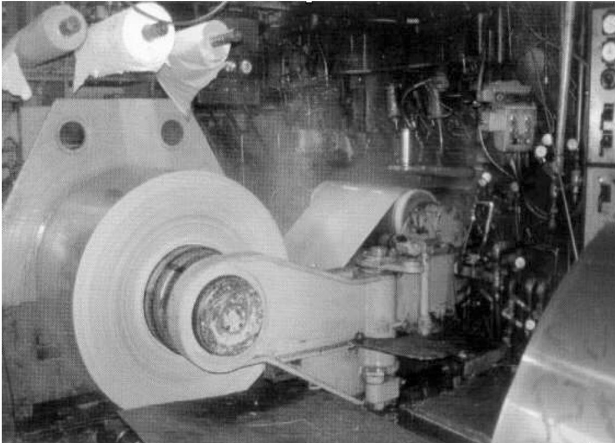
Figure 8.6: *Schematic of Reversing Mill*
