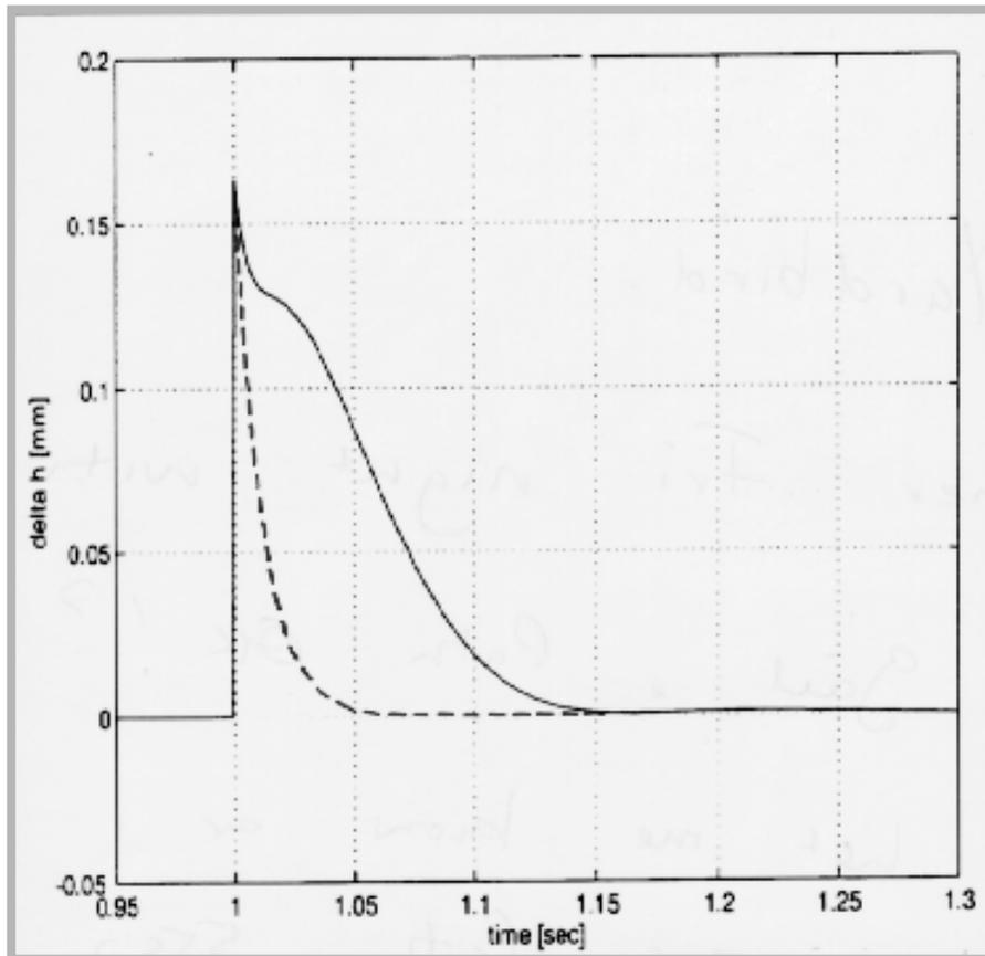
Recall that the solid line was the best that could be achieved with a single degree of freedom control whereas using feedforward we can achieve the dotted line.
