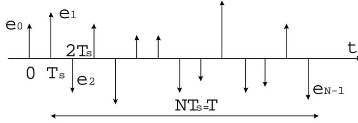
Fig. 3.1 Quantization noise sequence
