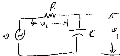
FOR THE CASE OF (b) & (c),  $\sigma = \infty \Rightarrow R = 0$ . HENCE, THE GENERATED EMF,  $v_2$  APPEARS ACROSS C. NOW, WE NEED TO TAKE INTO ACCOUNT THE VOLTAGE DROP IN CONDUCTORS.
