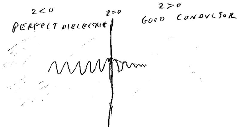
CONSIDER AN EM WAVE IMPINGING ON ~~THE~~ A GOOD CONDUCTOR FROM A PERFECT DIELECTRIC. LET THE BOUNDARY SURFACE
