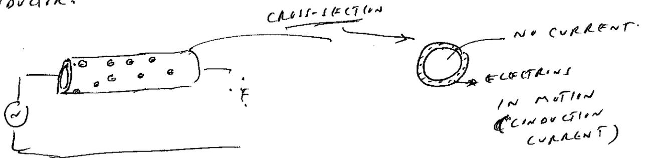
NOTE THAT THE ELECTRIC FIELD INTENSITY DECAYS EXPONENTIALLY WITH DISTANCE (FROM THE DIELECTRIC-CONDUCTION BOUNDARY). THIS LOSS OF ENERGY OF THE EM WAVE CORRESPONDS TO THE GAIN OF ENERGY OF ELECTRONS (KINETIC ENERGY). THE ELECTRIC FIELD INTENSITY IS THE FORCE PER +VE UNIT CHARGE.
